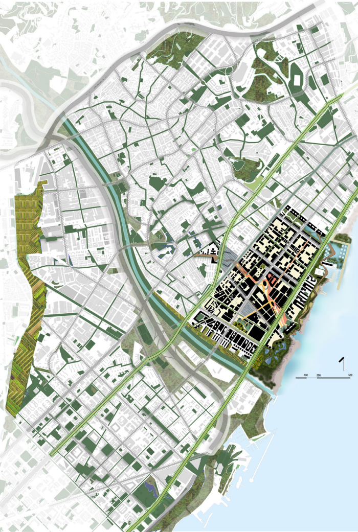
Perimeter scale map reflecting the newly defined mobility network,altered street systems and the contemporary production zones. The proposal highlights the conversion of industries into green industries while the streets are continuas green corridors for a low carbon,car lite district.
